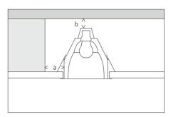
Installation of recessed luminaires according to the Furopean standard (EN 60598): the minimum distance a between the sides of the luminaires and building surfaces must be 50-75 mm. Between the upper surface of
